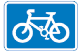
Diag 967: 'Route recommended for pedal cycles on the main carriageway of a road'
